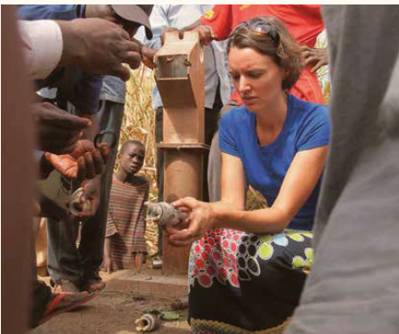
Top left: the whole community must help in the construction of new wells. Bottom left: Joanne shows the well committee the petrified rubber seal that stopped this pump from working for 15 years.
